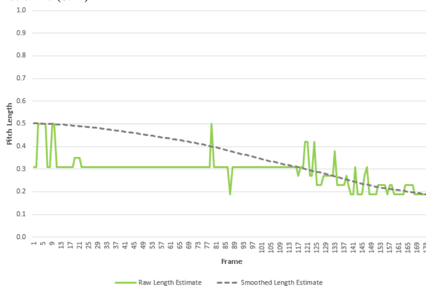
Figure 2: Raw length estimate per frame with loess smoothing for the length estimate overlaid for a kick-off.
